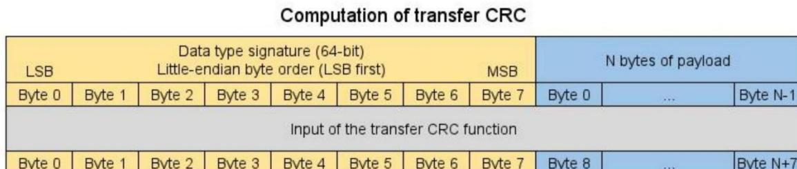
Note: The CRC calculation method with data signature is as shown in the diagram above. Add a
