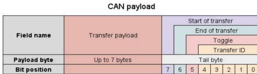
Some data packets may have valid data that exceeds 7 bytes. The TM-UAVCAN protocol specifies that data frames of up to 7 bytes use the Single Frame Transfer format, while data frames exceeding 7 bytes use the Multi-Frame Transfer format. Below are the definitions of Single Frame Transfer and Multi-Frame Transfer.
